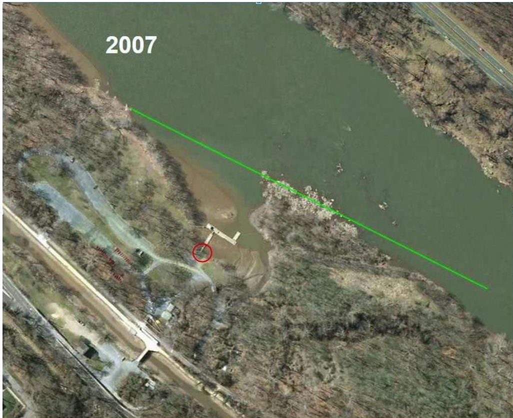
23-24. Siltation Threat to Cove; Fill Area (bottom right) Blocks High Water Scouring
